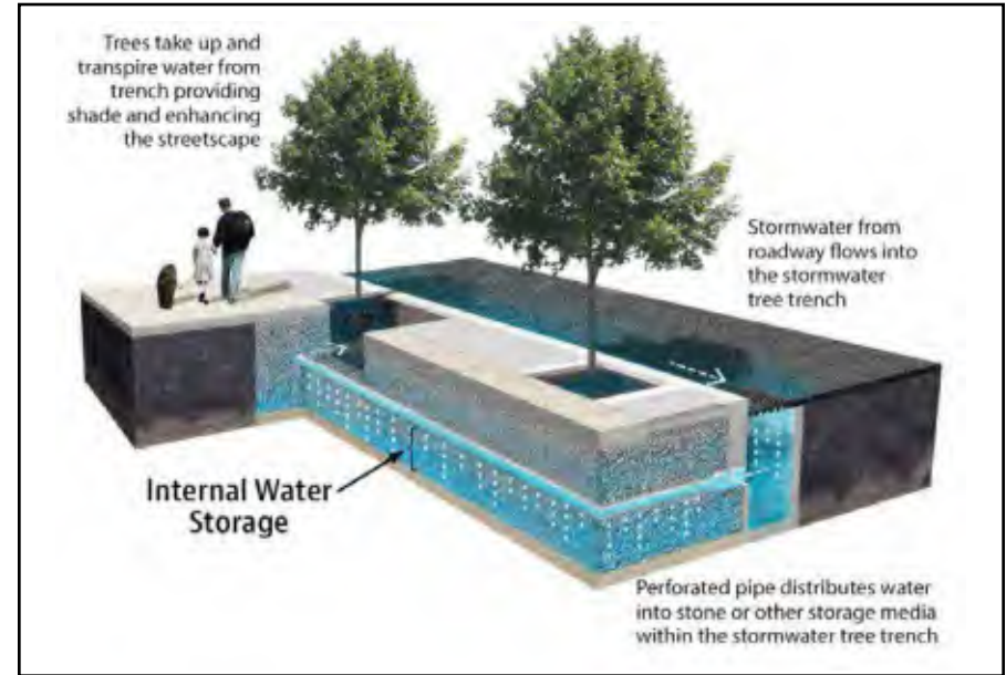
Design schematic for a stormwater tree trench.
